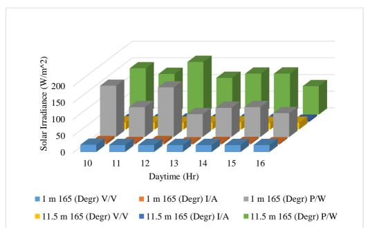
Figure 6d: Comparison of voltage, current, and power datasheet for 165° tilt angles at 1 m and 11.5 m.
