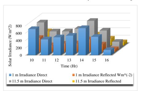
Figure 3: Direct and reflected irradiance at 1 m and 11.5 m on a sunny day.
