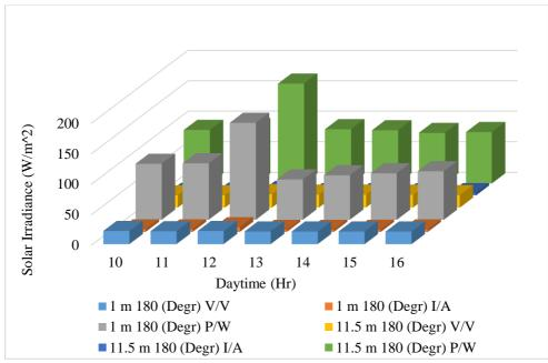
Figure 6e: Comparison of voltage, current, and power datasheet for 180° tilt angles at 1 m and 11.5 m.
