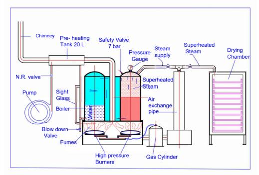
Figure 3: A schematic diagram of the low-pressure superheated steam dryer and associated units.
